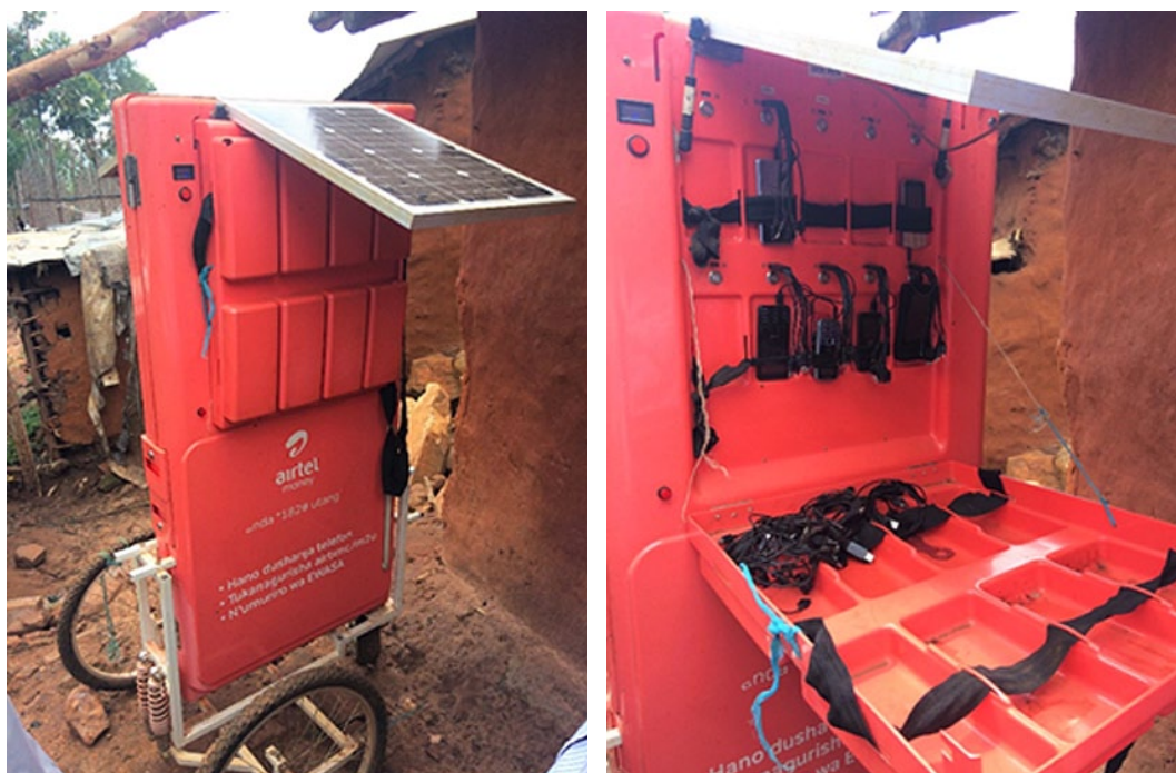
Solar powered phone charging shop in Nyabiheke refugee camp, Rwanda. Credit: S Rosenberg-Jansen
